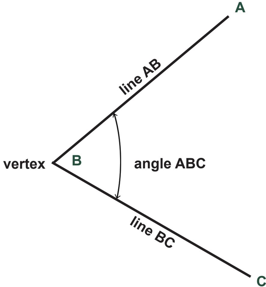
This picture shows how **angle ABC** is created when **line AB** and **line BC** intersect. **Vertex B** is the point where the two lines intersect.
